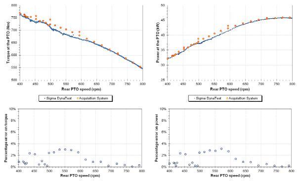
errors down to about 2 %, further rising the reliability of the acquisition system, which recordings can be considered substantially equal to the acquisitions made by the Sigma DynaTest.
