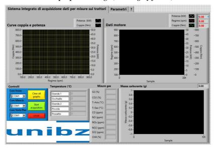
Fig. 6. Main tab of visual interface of "TRA-LOG" system; in the bottom-left angle there is the control panel (namely "*Controlli*") with the necessary items (drop-down menus, buttons) usable by the operator, while the remaining part of the screen is used to visualized the acquired signals
