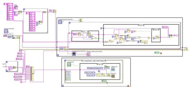
Fig. 5. Block diagram of integrated system, parts of it in charge of processing data-flow from gas analyser (*top grey frame*) and creating file in which saving all data with proper headings (*bottom grey frame*)
