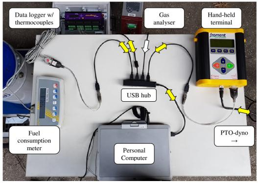
Fig. 2. Wiring layout of different instruments connected together to compose integrated acquisition system (NB: PTO-dyno is outside the photograph); the white/yellow arrow indicates a unidirectional/bidirectional flow of signals in that wire
